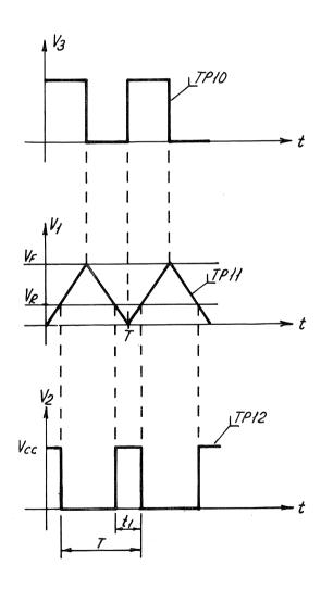
$V_2$  is mean value rectified (R321a, C320) and then fed to the meter amplifier (IC307c). The meter amplifier inverts the mean value, so when  $V_{CC} \times \frac{V_R}{V_F} = 0$  then the output voltage is 13.5V and when  $V_{CC} \times \frac{V_R}{V_F} = V_{CC}$  the output voltage is zero.
