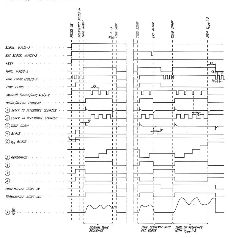
$38mS < t_1 < 163mS$   $25mS < t_2 < 108.8mS$   $3s < t_3 < 7s$   $0.5mS < t_4 < 2mS$
