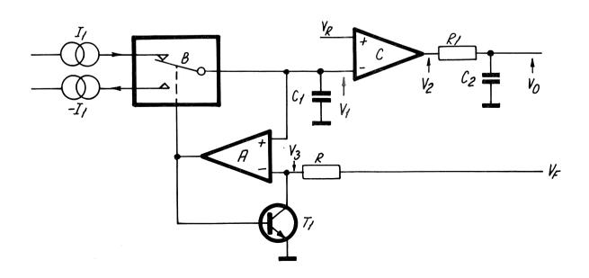
C1 is charged (IC316b, T317) or discharged (IC316a, T316) with a constant current, depending on the position of the analog switch B (IC317) which is controlled by the comparator A. When V1 is less than VF, C1 is charged with I1 until V1 = VF then B switches and C1 is decharged with -I1 and T1 is switched on. C1 is decharging until V1 = 0. V1 is now a triangle wave with a periode time T depending on VF, T =  $\frac{2 \times VF \times C}{I1}$  (see wave forms below).
